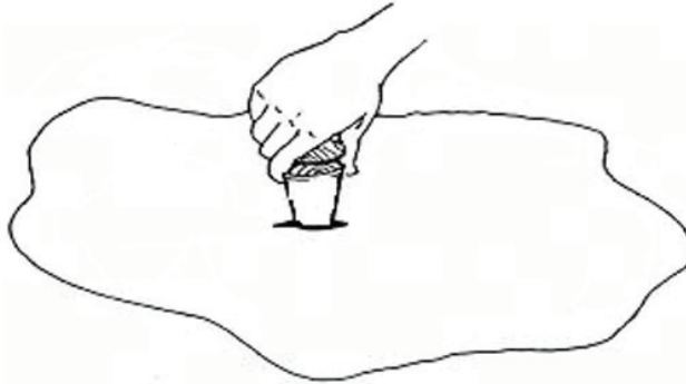
Figure 2. Wood Plug Installation.
